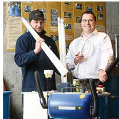
The USEPA-approved fluorescent light bulb crusher operated to fill forty-four gallon sealed drums with the mercury containing waste for shipment and recycling.
