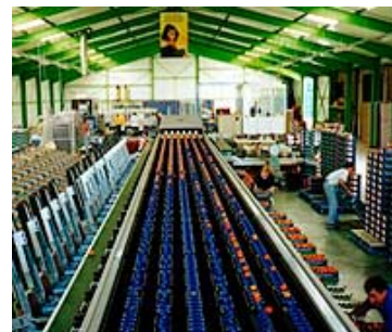
Compac Sorting Equipment's high-speed conveyor belt for weighing fruit, which was refined with input from Massey industrial mathematicians.
